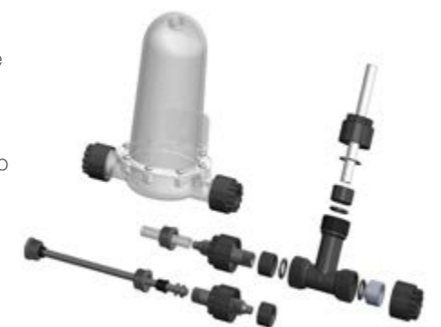
Exploded View of Large Bore Fittings Range
